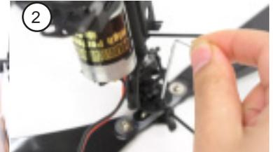
3. Adjust the blade tension on the main rotor grips to be equal using a phillips head screwdriver. The tightness should be snug but should also allow the blades to move. Setting the blades too tight may contribute to vibration.
