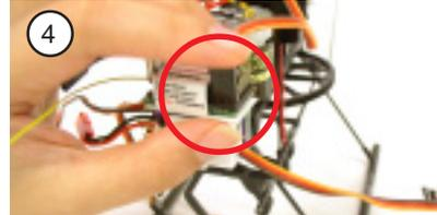
4. Plug in channel 1 for aileron servo.
