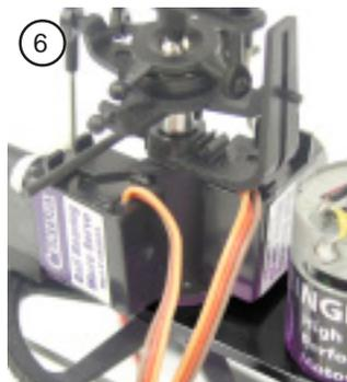
4. Once the mounting position of the servo is determined carefully mount the servo to the mast tower. If the servo has a label on the same side that will mount with double sided tape, peel off the label and clean the surface using rubbing alcohol.
