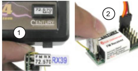
2. Note that all electronics plug into the receiver with the wires as pictured (orange wire faces receiver label). Follow the diagram for each electronic connection. Once the electronics system is connected and the transmitter is turned on, follow this step-by-step process to check your equipment.
